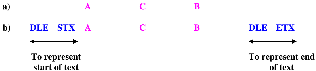
Figure 3.1.13 Character Oriented (a) Data to be send to the peer, (b) Data after being character stuffed
