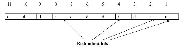
Figure 3.2.8 Positions of redundancy bits in hamming code
