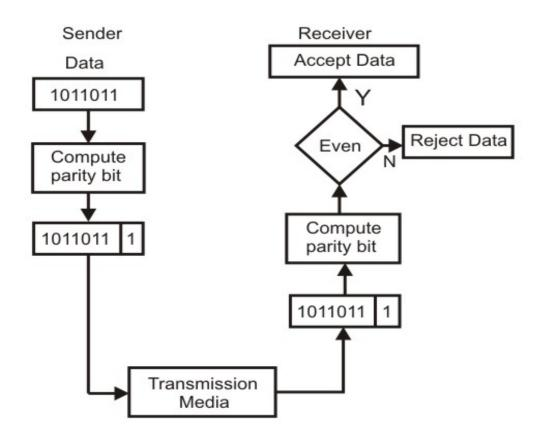
Figure 3.2.3 Even-parity checking scheme
