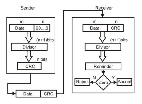
Figure 3.2.6 Basic scheme for Cyclic Redundancy Checking
