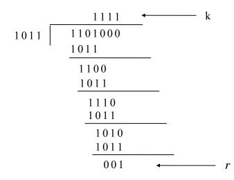
Figure 3.2.7 Cyclic Redundancy Checks (CRC)
