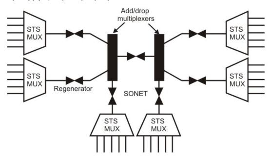
Figure 4.3.1 Devices used in the SONET system
