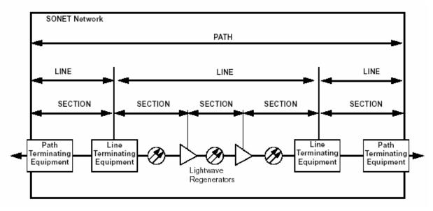
Figure 4.3.2 Section, line and path in a SONET network
