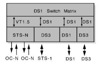
Figure 4.3.6 Wideband digital cross-connect
