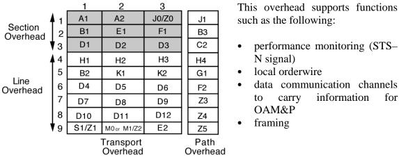
Figure 4.3.8 Section Overhead
