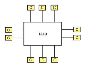
Figure 5.3.5 Interfacing a computer in 10Base-T standard
