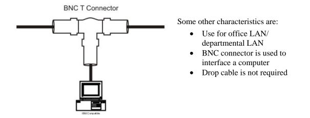
Figure 5.3.4 Interfacing a computer in 10Base-2 standard
