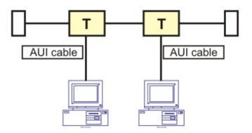
Figure 5.3.3 Interfacing a Computer in 10Base-5 standard
