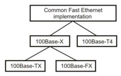
Figure 5.6.2 Fast Ethernet implementations
