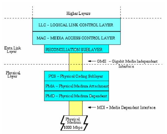
Figure 5.6.7 Gigabit Ethernet Architecture-2
