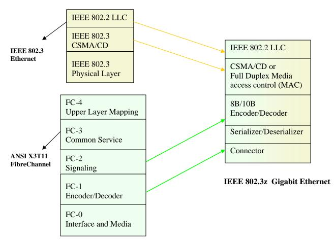
Figure 5.6.6 Gigabit Ethernet Architecture -1
