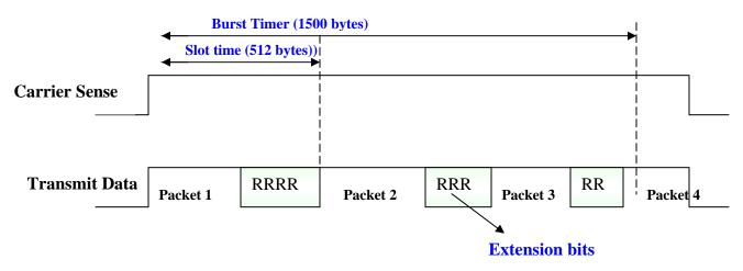
Figure 5.6.9 Packet Bursting
