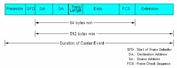
Figure 5.6.8 Ethernet Frame Format With Carrier Extension
