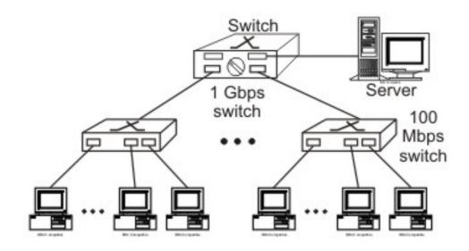
Figure 5.6.11 Migration to Gigabit Ethernet Backbone network
