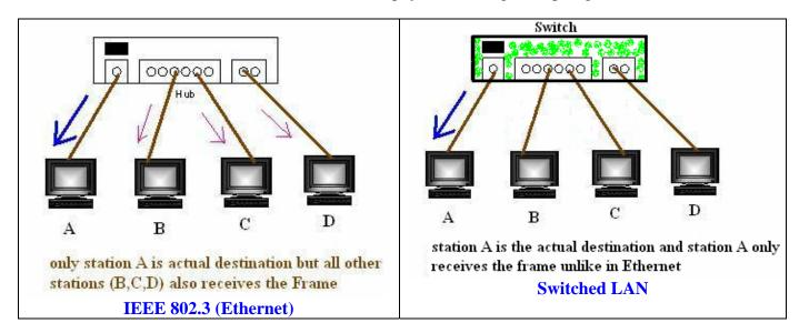
Figure 5.6.1 Difference Between 802.3 and Switched LAN
