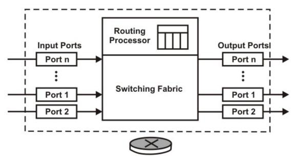
Figure 6.1.13 Schematic diagram of a router
