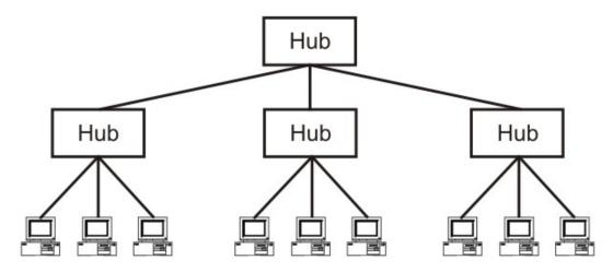
Figure 6.1.3 Hub as a multi-port repeater can be connected in a hierarchical manner to form a single LAN with many nodes
