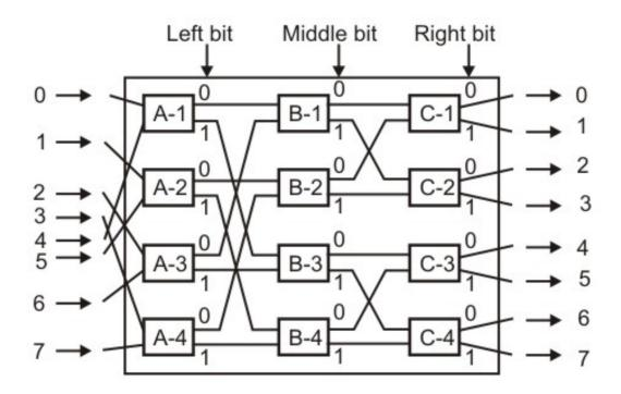
Figure 6.1.15 Switching fabric of a router
