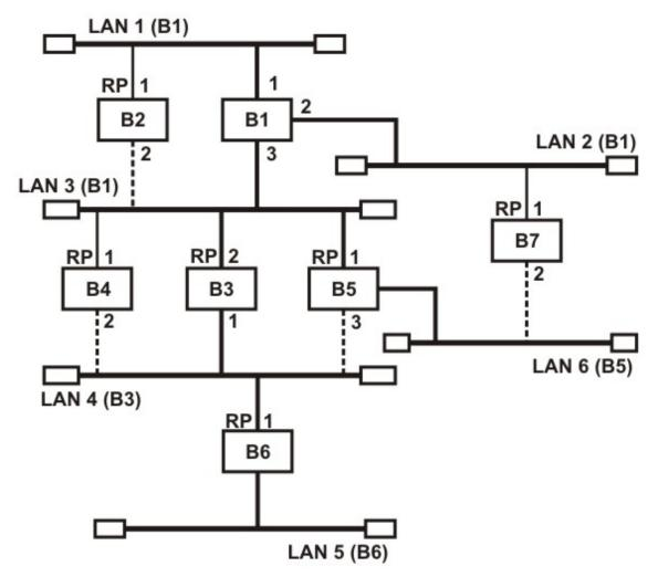
Figure 6.1.10 Spanning tree of a network of bridges
