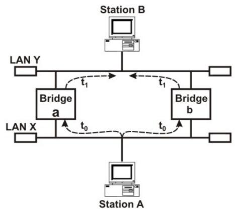
Figure 6.1.9 Loop problem in a network using bridges
