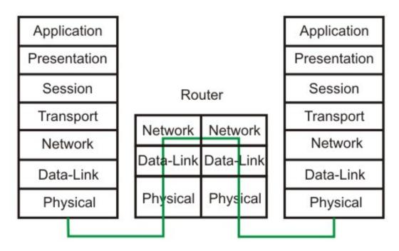
Figure 6.1.16 Communication through a router
