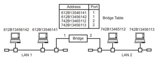
Figure 6.1.4 A bridge connecting two separate LANs
