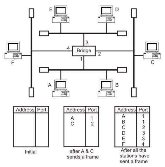
Figure 6.1.8 Creation of a bridge-forwarding table
