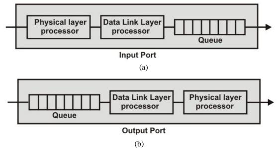
Figure 6.1.14 Schematic diagram of a router
