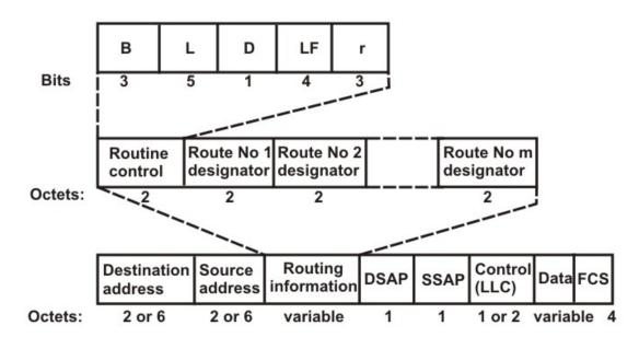
Figure 6.1.11 Source routing frame
