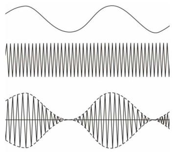
**Figure 2.5.4** (*b*) Envelope of the signal  $1+m e_m(t)$  for m = 1
