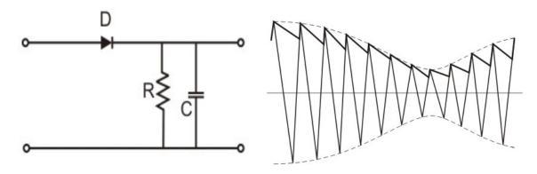
Figure 2.5.10 Recovery of the baseband signal using envelope detection
