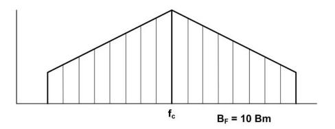
Figure 2.5.13 Bandwidth of a frequency modulated signal
