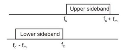
Figure 2.5.9 Single Sideband (SSB) Modulation
