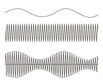
**Figure 2.5.4** (*a*) Envelope of the signal  $1 + m e_m(t)$  for m < 1
