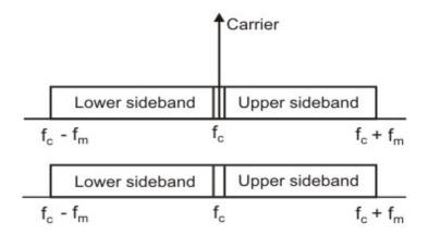
Figure 2.5.8 Double-Sideband with Suppressed Carrier (DSBSC) Modulation
