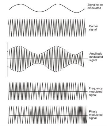
Figure 2.5.15. Analog data to Analog signal modulation techniques at a glance
