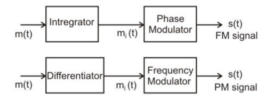
Figure 2.5.14 Difference between frequency and phase modulation
