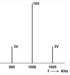
Figure 2.5.6 Spectrum of the modulated signal of the above example
