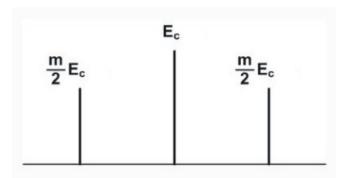
Figure 2.5.5 Spectrum of a modulated signal
