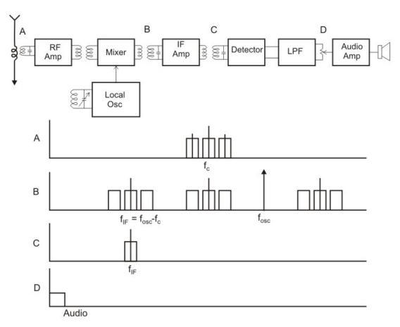
Figure 2.7.11 Operation of a superheterodyne AM radio receiver
