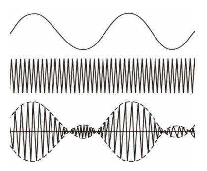
**Figure 2.5.4** (*c*) Envelope of the signal  $1+m e_m(t)$  for m > 1
