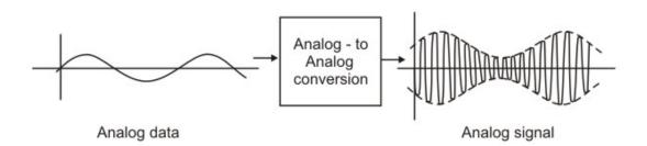
Figure 2.5.1 Translation of analog data to analog signal
