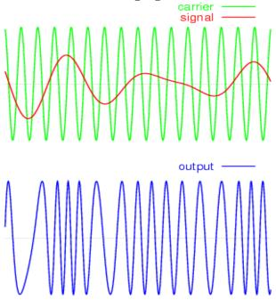
Figure 2.5.12 Angle modulation
