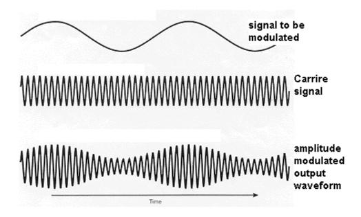
Figure 2.5.3 Amplitude Modulation
