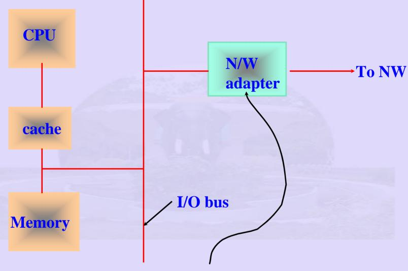
A device that transfer data between workstation memory and NW link
