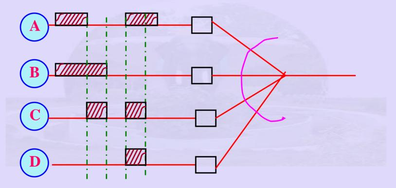
Asynchronous TDM: Intelligent TDM – allocate time slots on demand
